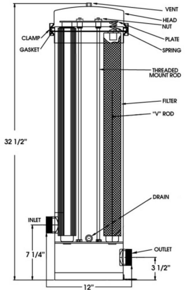
12. Securely screw bleed off valve with pressure gauge into place onto lid of housing using teflon tape. Securely screw the 1/2" NPT 1/4 turn water spigot and threaded plug into openings at the base of the housing. Use teflon tape on threads with pipe dope.
