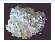
Aragonite, another form of calcium carbonate, has very different characteristics to calcite. When calcium carbonate precipitates as argonite it forms a non-adhering harmless insoluble crystal that is either consumed or carried through the system to the drain.
